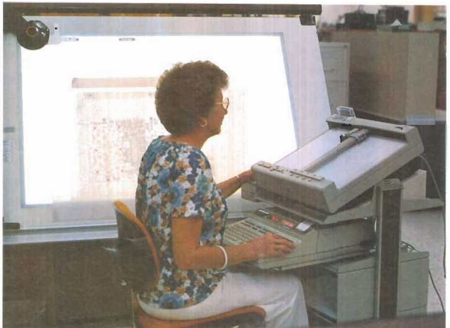
Mel Lester of the PC manufacturing group operates the 9872A to generate a drawing. Controls for the track ball device added to the 9872 are visible at the far side of the plotter.
