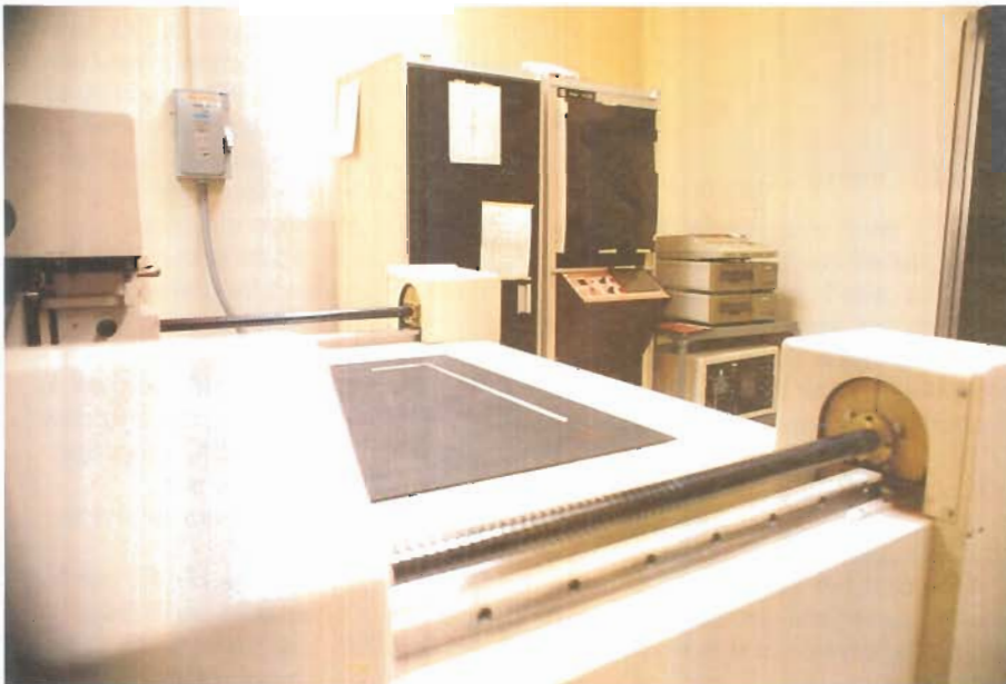
Once the Digiplot program has been completed, data is relayed to the department's Model 33B Gerber Photoplotter, which produces the high-accuracy negatives used in producing PC boards.
