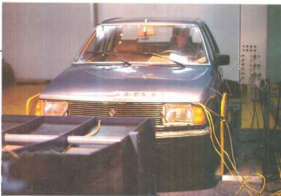
Researchers test a Solex intake system on a dynamometer in a climate-controlled test chamber.
